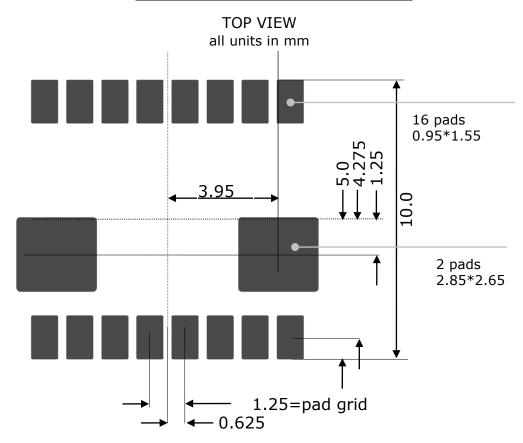
Note: For prototyping, GNS3301B is available on a stamp design adaptor board. Recommended mainboard pad layout will fit for both.
