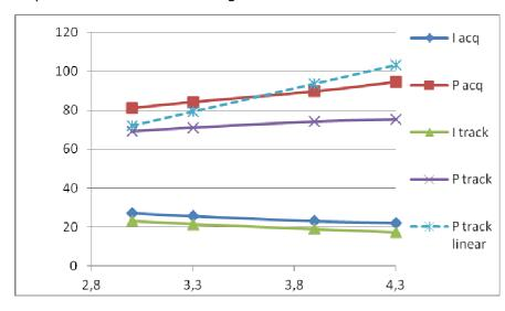
Note: values are measured in stable states after 15 min operation. Tracking with 6 SVs in solution at - 130dBm
