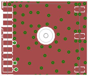
The ground plane can be part of the main ground layer of the mainboard, some (small) components in the neighborhood are acceptable. Do not place any bulky or metallic components near the antenna (in a distance below 30mm) to avoid unwanted electromagnetic shielding effects. It's recommended to place GNS601uLP near the rim of the main PCB, so that the antenna has a wide unobstructed working angle.
