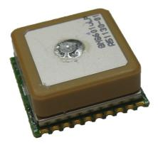
The navigation performance and accuracy is improved by using correction data from SBAS (WAAS, EGNOS, GAGAN, MSAS), QZSS.
