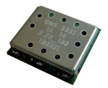
The low power design makes it easy to implement this module in power sensitive, battery supplied applications. Very low power requirements (typ. 72mW@ 3.3V) and internal voltage regulator makes it easy to run the module with various power supplies and allows direct connection to LiIon batteries.
