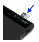
Turn the GNS power switch on-off-on within 1.5 seconds (same procedure as start logging)
