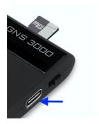
5. Insert micro-SD card into the GNS 3000
