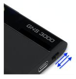
After successful firmware update the three GNS 3000 LEDs will blink three times.
