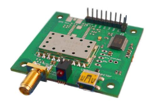
The GNS 5851 StarterKit has been designed to support developers during design-in of the GNS 5851 stand-alone module solution.
